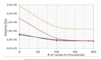
The <u>elasticity module</u> shows how much pressure you need to apply with your cutting machine for the same ejection capabilities compared to US sheets.
