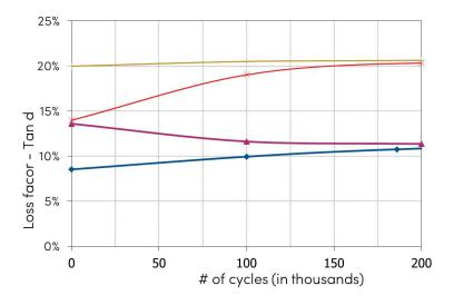
Although difficult to calculate, interpreting the <u>loss factor</u> is straightforward: when you compress the rubber, you give it energy to bounce back. But the loss factor shows you what you are not getting back!
